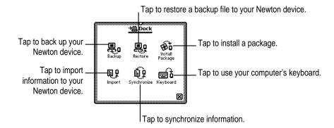
The connection utilities work the same way on your Newton device as on your computer, with the exception of export. To export information from your Newton device, you must use the Newton Connection Utilities window on your computer. When you use the Newton device to initiate synchronization with your computer, the utilities use the settings on your computer. Use the Newton Connection Utilities on your computer to changes these settings, if necessary.
