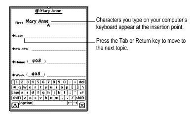
You can use all standard alphabetic and numeric keys on your keyboard to enter information on your Newton device. You can also use the Tab and Return keys to move between topics. Special keys, such as F1, are not supported.
