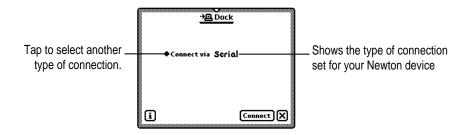
2 If necessary, tap "Connect via" to change the type of connection and choose Serial.
