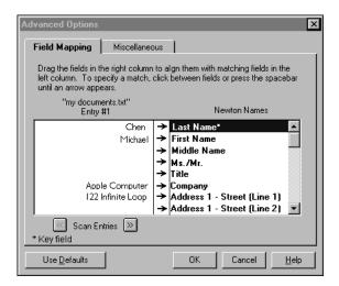
Instead of field names, one column shows entries in the file you're importing. You can move backward and forward through entries in the file by clicking the Scan Entries buttons.
