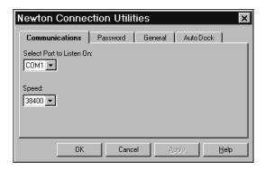
3 Select the COM port to which the Newton's serial cable is connected, using the "Select Port to Listen On" drop-down list.
