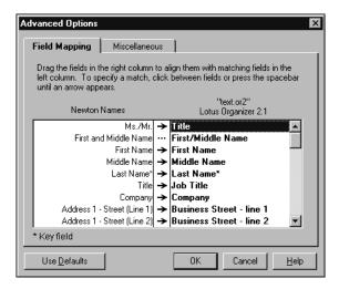
One column lists the application you're transferring information from (the source application). The other column lists the application you're transferring information to (the target application). The middle column of arrows shows which fields of information will be transferred.
